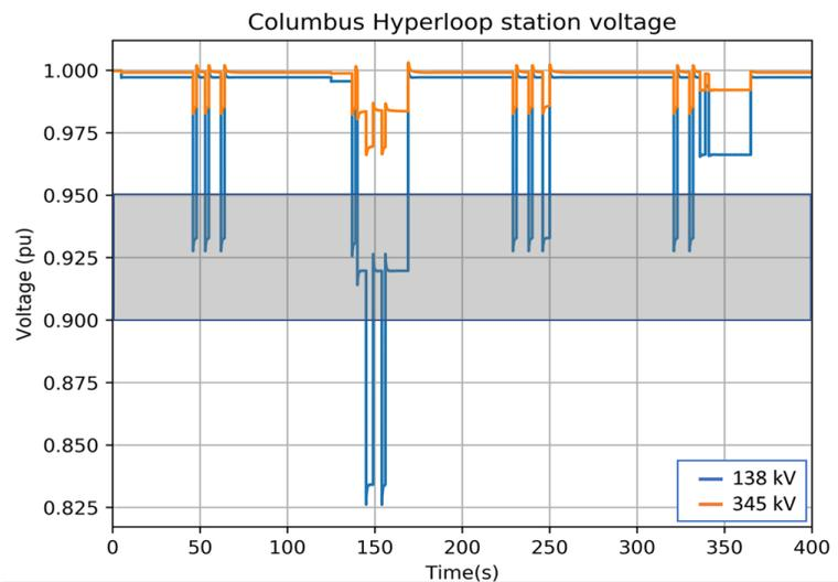
The shaded box represents the range of typical voltage violation thresholds. 0.95pu is typical for normal operation and 0.90pu is typical for contingency situations.
