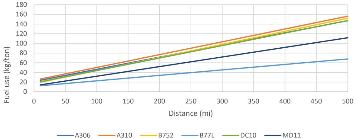
Figure 21: Fuel use by aircraft, estimated using the algorithm and input values from O’Kelly 2014.
