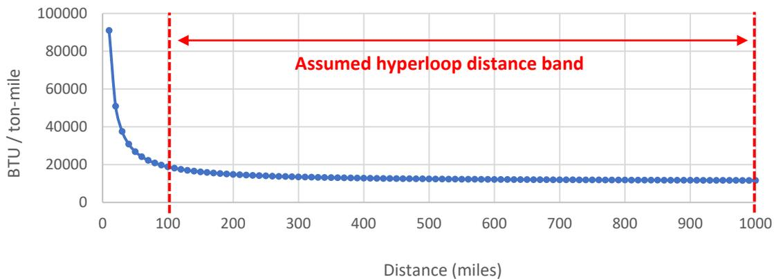
Figure 22: Relationship between air freight energy intensity and distance shipped.
