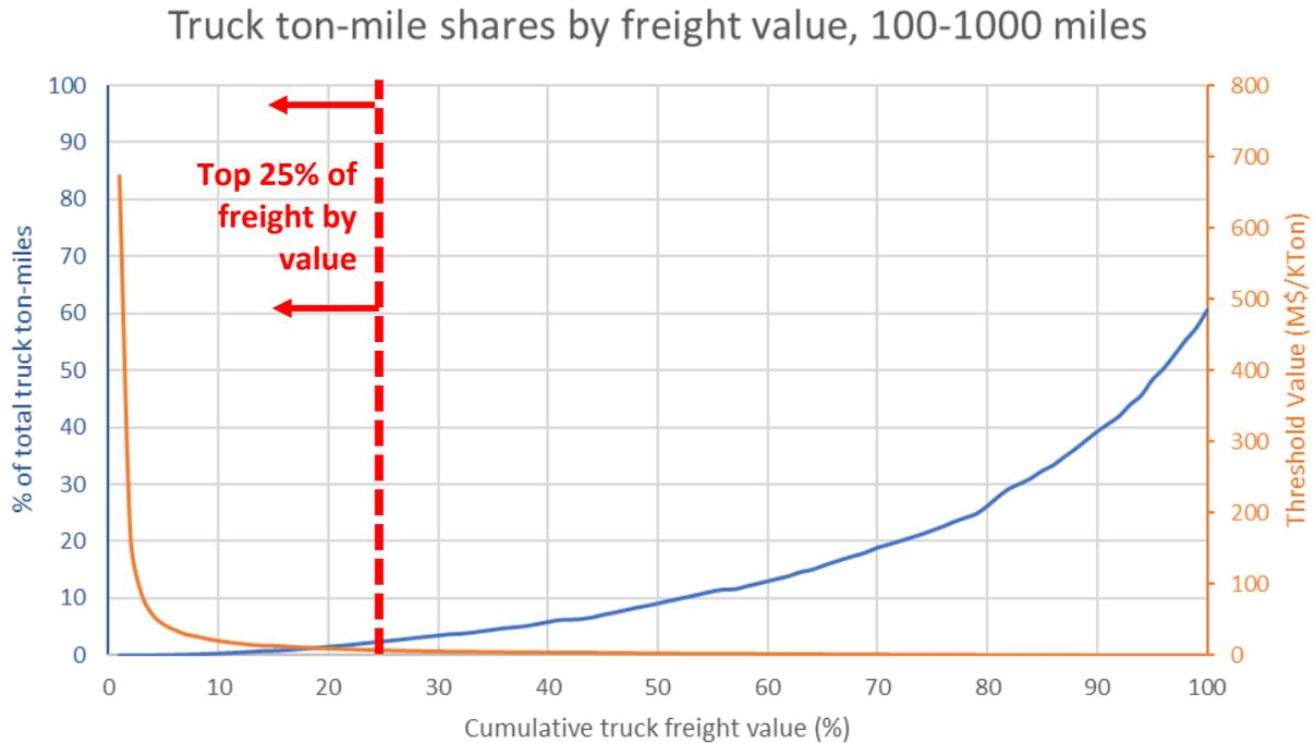
Figure 20: Analysis of truck freight demand by freight value (Source: Analysis of FAF data)<sup>89</sup>
