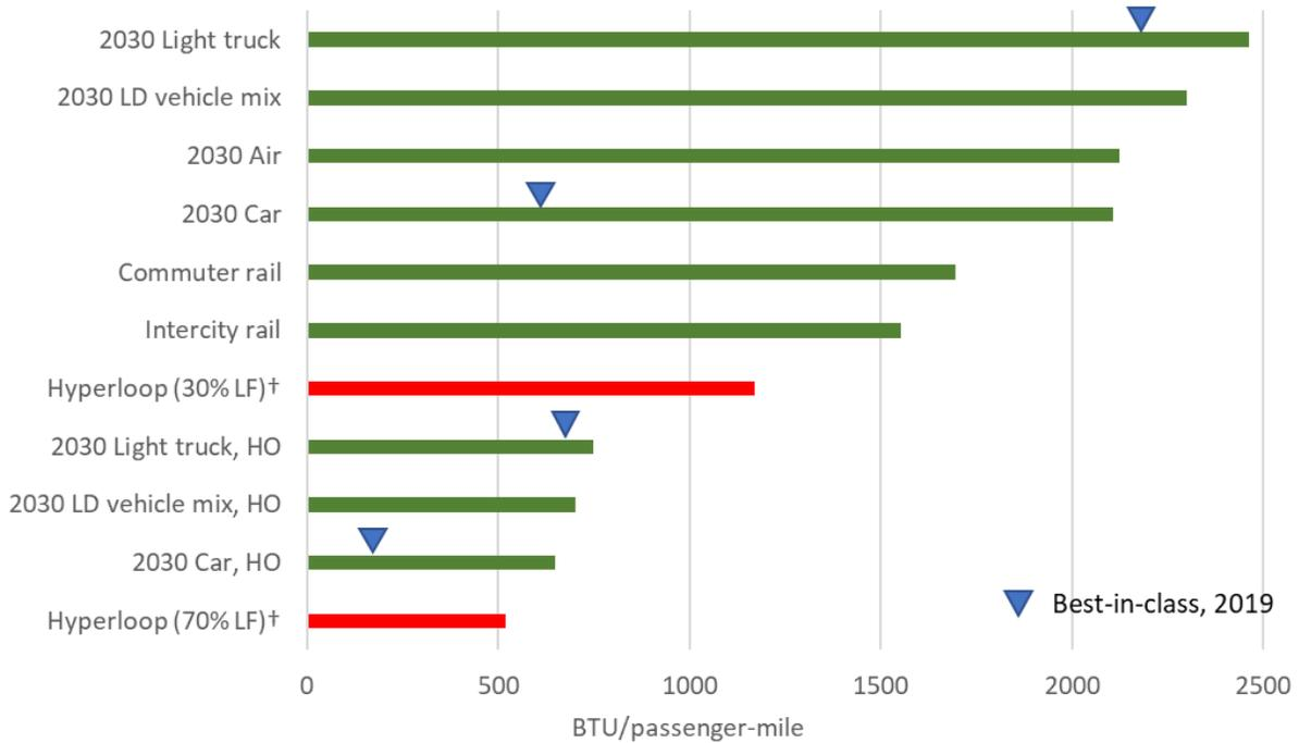
Figure 14: Comparison of energy intensity by transportation mode. BTU = "British Thermal Units", a standard measure of energy. LF stands for Load Factor and HO stands for High Occupancy.<sup>61,62</sup>
